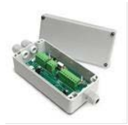
DSJ1 & 4 Strain gauge data converter to RS232. Modbus, CAN, RS485 available as single or 4 channel IP65 enclosure
