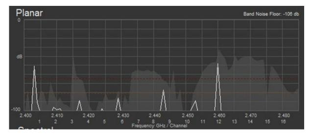
This shows a good RF environment. The Band Noise Floor is low and there are no red traces indicating that there are plenty of signal free gaps to enable T24 to transmit. There is traffic across the whole band with higher signal traffic between channels 11 to 15, but there is nothing that would affect T24 operation.
