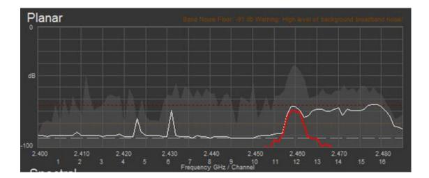
This shows how the display would look if the band noise floor slowly crept up. The red trace is only visible on channel 12 but other channels that were once OK (Having a very low minimum signal level) now have a viewable level of minimum signal noise. A double-click on the planar chart would reset the peak and minimum calculations so the minimum red trace would then follow the more recent higher noise floor – see image on next page.
