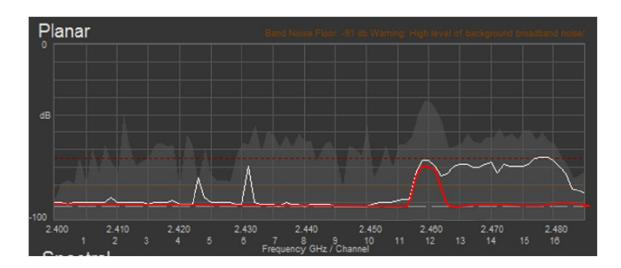
Whilst you are doing this, it is a very good idea to take screen shots of the whole window (the spectral view can give a useful history as well). This will be a useful record and could help Mantracourt with fault finding. It will also be useful to note down what the noise floor was as this could limit the possible range.
