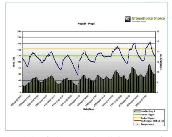
Figure 1 - Example of remote data of strut load, temperature and load warning trigger
