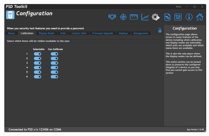
This section allows you to configure the available six calibration ranges availability from the menu and whether the range is selectable via the keypad (If that keypad action has been enabled).
