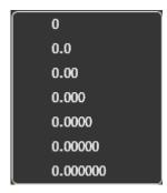
Note that the decimal places can also be modified (globally for the currently displayed engineering units) by using a long press on the keypad left and right direction keys (If this action has been allowed).
