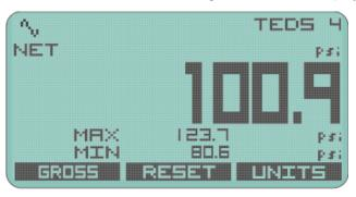
Soft keys allow you to toggle between Zeroed and Gross values and to Reset the min and max to the current value. The usual Units selection is also available.
