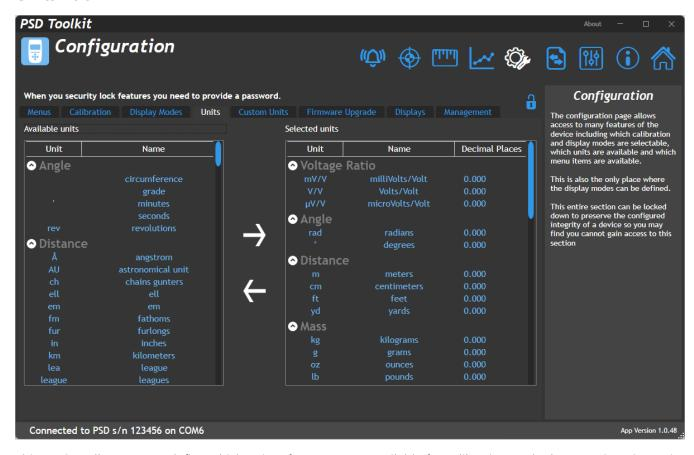
This section allows you to define which units of measure are available for calibration as the base engineering units and also any unit conversions that are selectable from the Units soft key that appears on most display modes. Two lists are displayed. The left one shows all available units that are *not* currently enabled and the one on the right shows the units that are available for calibrating or conversion.
