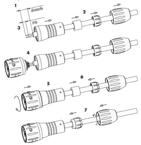
If a cable is already connected to the connector remember to unscrew the cable clamp before unscrewing the main body of the connector otherwise, you risk twisting the cable and breaking the connections. If the main body is difficult to unscrew it may be easier to lock the connector to the handheld then grip and unscrew the main body in an anti-clockwise direction.
