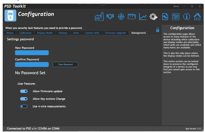
Access to the entire set of Configuration settings can be locked with a password. Without the password a user cannot change any of the protected settings which include the available Display Modes. This tab allows setting a new password or removing an existing password to protect or release the configuration settings.
