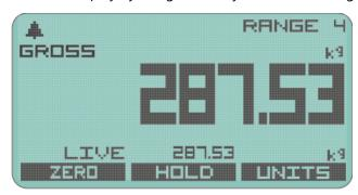
The other soft keys allow being able to Zero the main display or go back to displaying Gross. As usual there is a soft key to allow Units to be selected.
