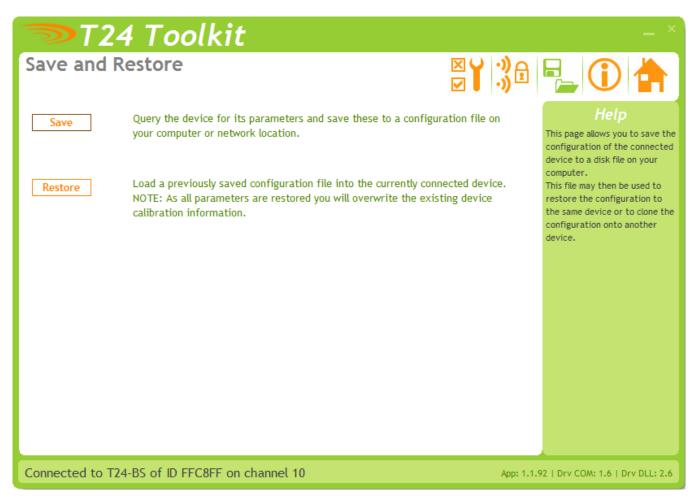
Here you can save the device settings to a file on your PC so that they can be later loaded back into the same or different module.
