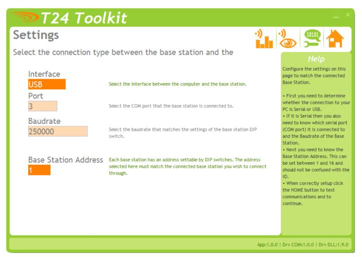
Select the required interface type and base station address.
