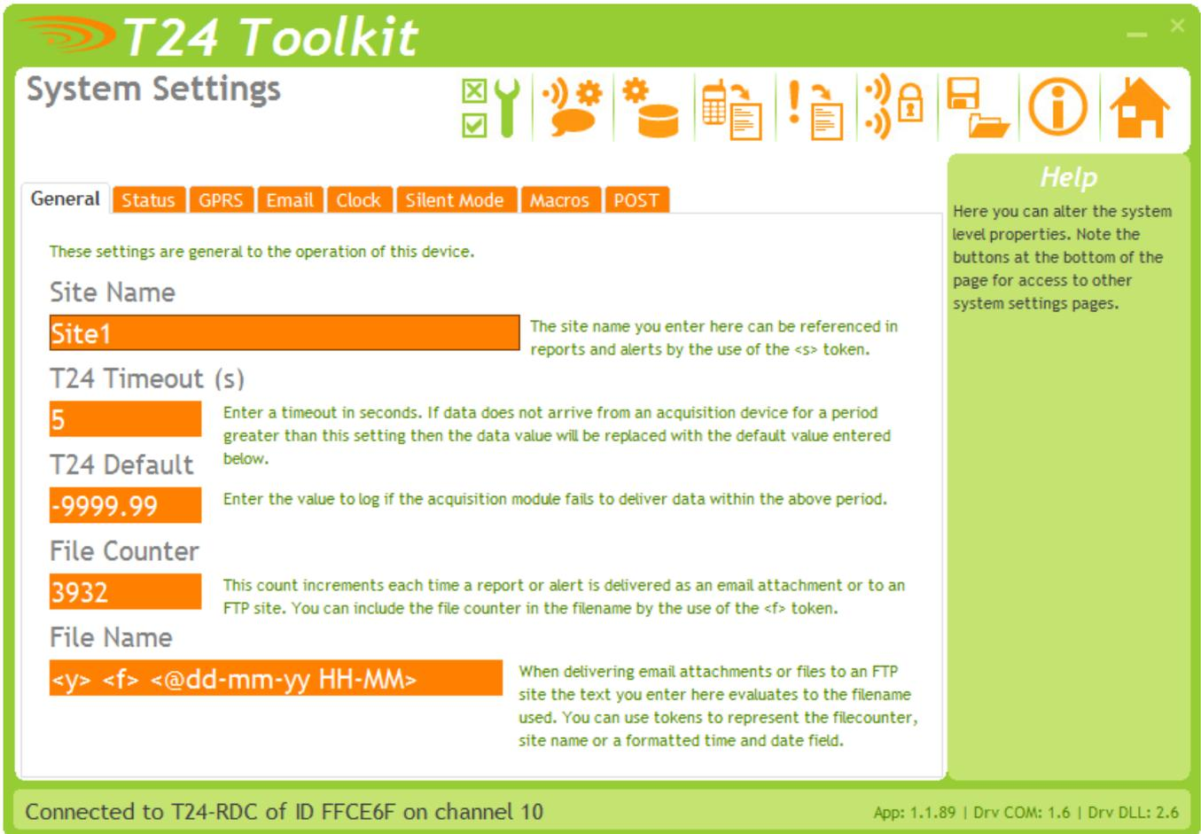
This is where much of the operation settings are configured. The parameters are split over multiple tabs. Just click a tab to move to the desired section. Changes made on this page are saved automatically.
