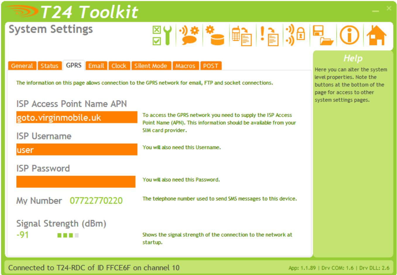
The settings here apply to the GPRS network and affect the delivery to FTP, email and sockets.
