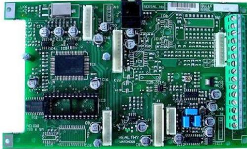
*Flexible digital signal conditioning amplifier for multiple or single load cell applications, offering very easy one-pass calibration and fast set-up*
