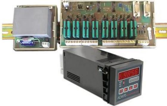
*The 12 Component Batch Weighing Controller adds the capability to manage and control up to 12 different components or ingredients, that can be combined into 10 separate menus (or products)*
