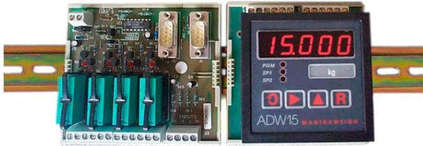
*The ADW-FFW Weighing Indicator is to control high speed, high accuracy filling by weight for strain gauge or load cell applications. Either in a stand alone mode or in conjunction with a PLC*
