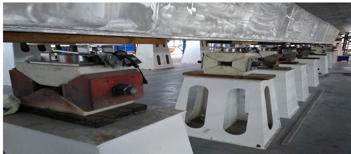
Load cells + mounting kits mounted on the boat supports
