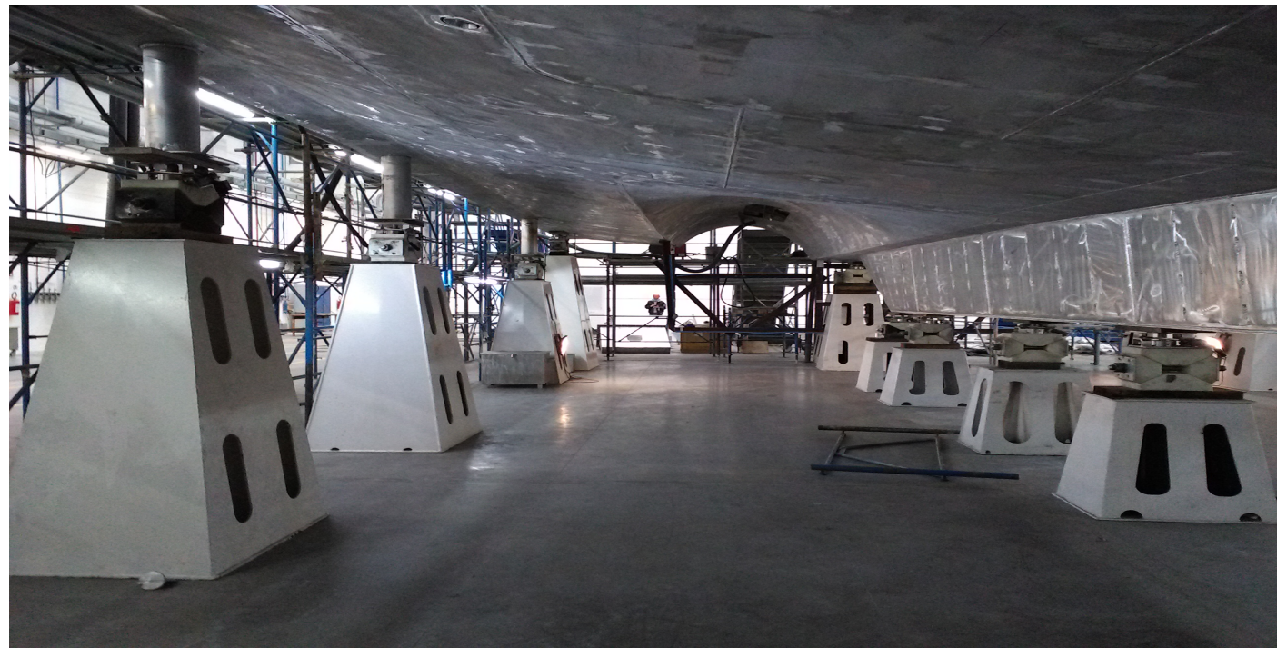
Load cells + mounting kits mounted on the boat supports
