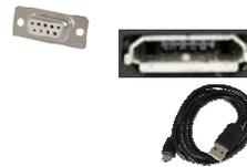
The new version of the DSCUSB has a D9 connector and a female micro USB connector. It is also supplied with a USB to micro USB cable.
