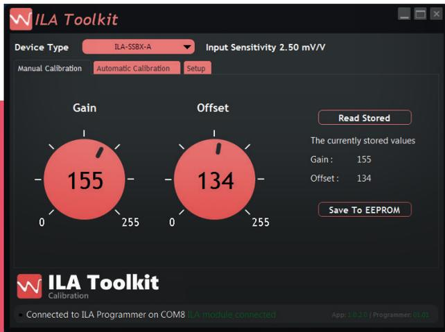
Manual calibration can simply be achieved by adjusting the virtual gain and offset potentiometers.
