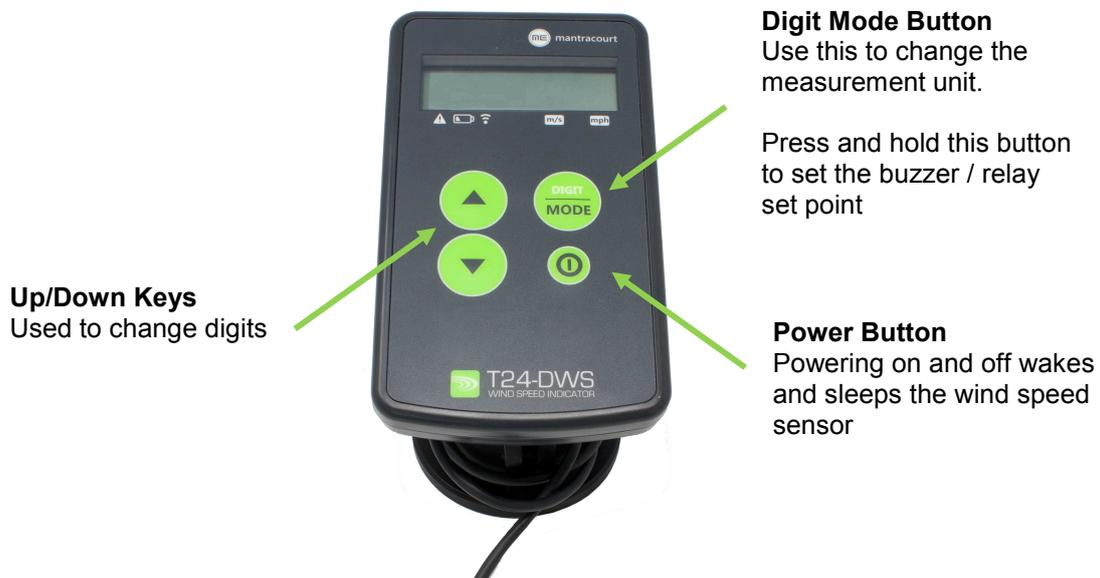
The **buzzer/relay set point** is set using the buttons on the display. Press and hold the **Digit/Mode** button until all seven digits are shown.
