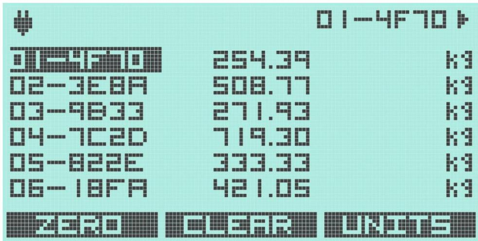
It is possible to scroll up and down through the list with the up and down keys and then move to a **Detail** display with the right arrow key.
