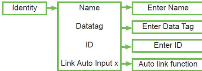
It is possible to auto populate the datatag and ID for the input using the Link Auto function. Activate this and follow the instructions on the handheld. The data tag and ID will be set and the transmitter will now be on the same radio settings as the handheld.
