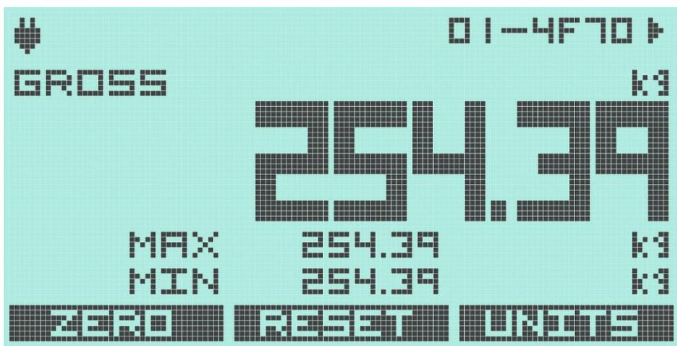
The user can also scroll up and down through the available transmitters in the detail display. The detail display allows a zero (tare) to be applied to that input channel and also shows the maximum and minimum values that have been seen for that channel.
