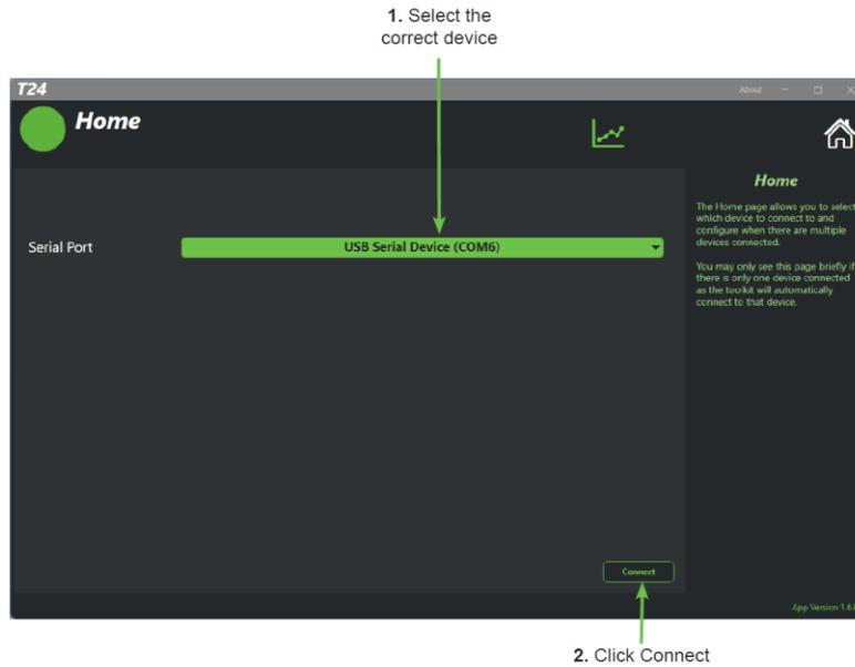
If only one T24-HK-S is connected, then the toolkit will connect automatically. Navigation is achieved using the icons along the top of the toolkit.
