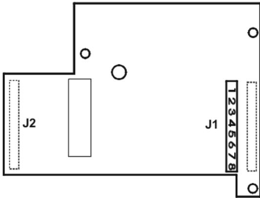
**Figure 4.6 Thermocouple Connectors**
