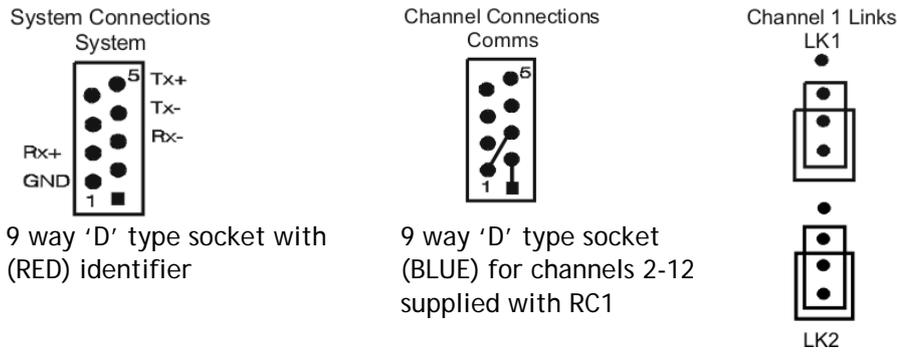
Figure 5.14 RC1 Baud Rate Selection
