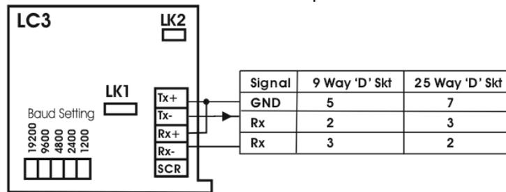
Figure 5.12 LC3 RS232 Mode Connection to Printer
