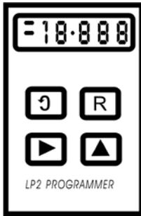
*Figure 2.14 LP2 Remote hand Held Programmer Unit (UAB)*
