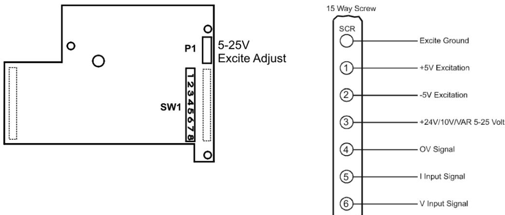
**Figure 4.2 The UALV1 - LVDT Module Rear Panel Connections**
