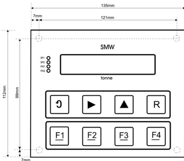
4mm M4 studs x 12mm for mounting. Sealing is provided by a Neoprene gasket
