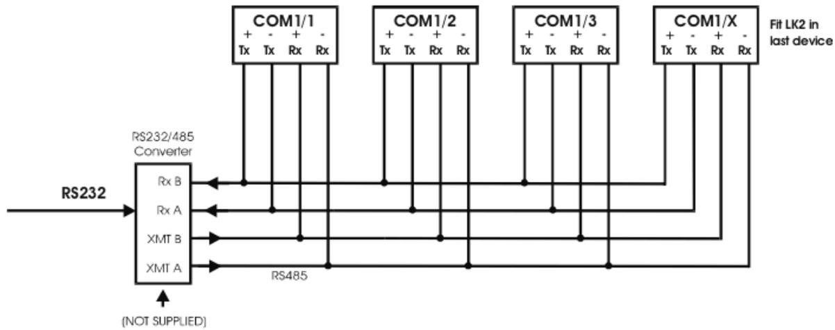
Figure 5.11 LC3 RS232 Mode Connection to PC
