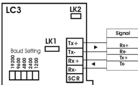
Figure 5.10 Connecting Multiple Units on RS485
