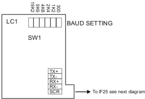
**Figure 5.8 IF25 Connecting Multiple Process Amplifiers**
