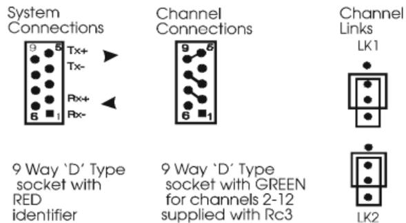
Note: The last device may be terminated by 120R resistor by fitting LK2 on RC3 module. LK1 on RC3 must not be fitted for multi-drop applications.
