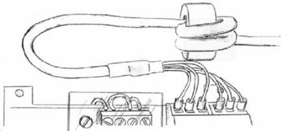
To meet the Specified EMC Fast transient requirements it is important that the ferrite ring supplied is fitted as per the following instructions.
