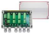
Photo showing the DSJ4 fitted in an optional ABS surface mounting case.
